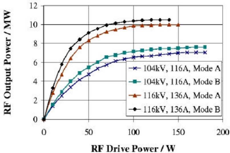
Fig.7 : RF output power as function of RF drive power of the MBK 2 at 0.5 ms pulse duration
