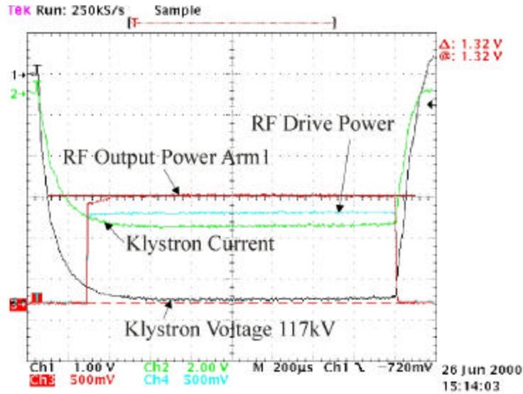
Fig 6: Waveforms at 10MW output recorded on MBK1
