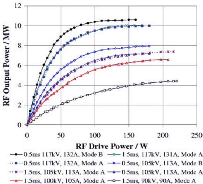
Fig5: RF output power as function of RF drive power of the MBK 1
