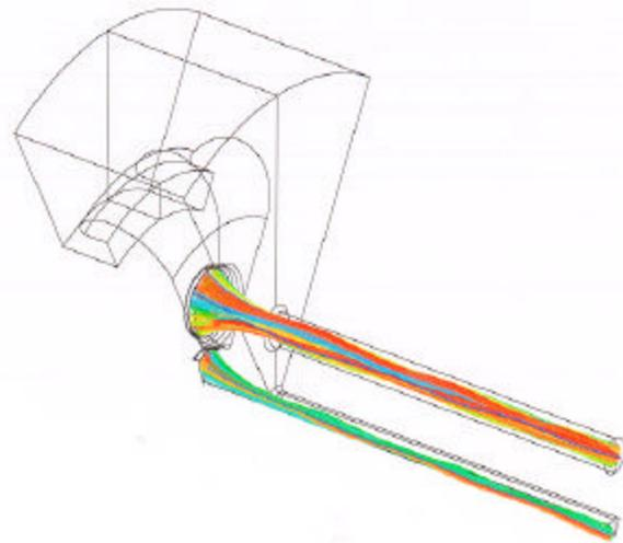
Fig. 3 Electron trajectories
