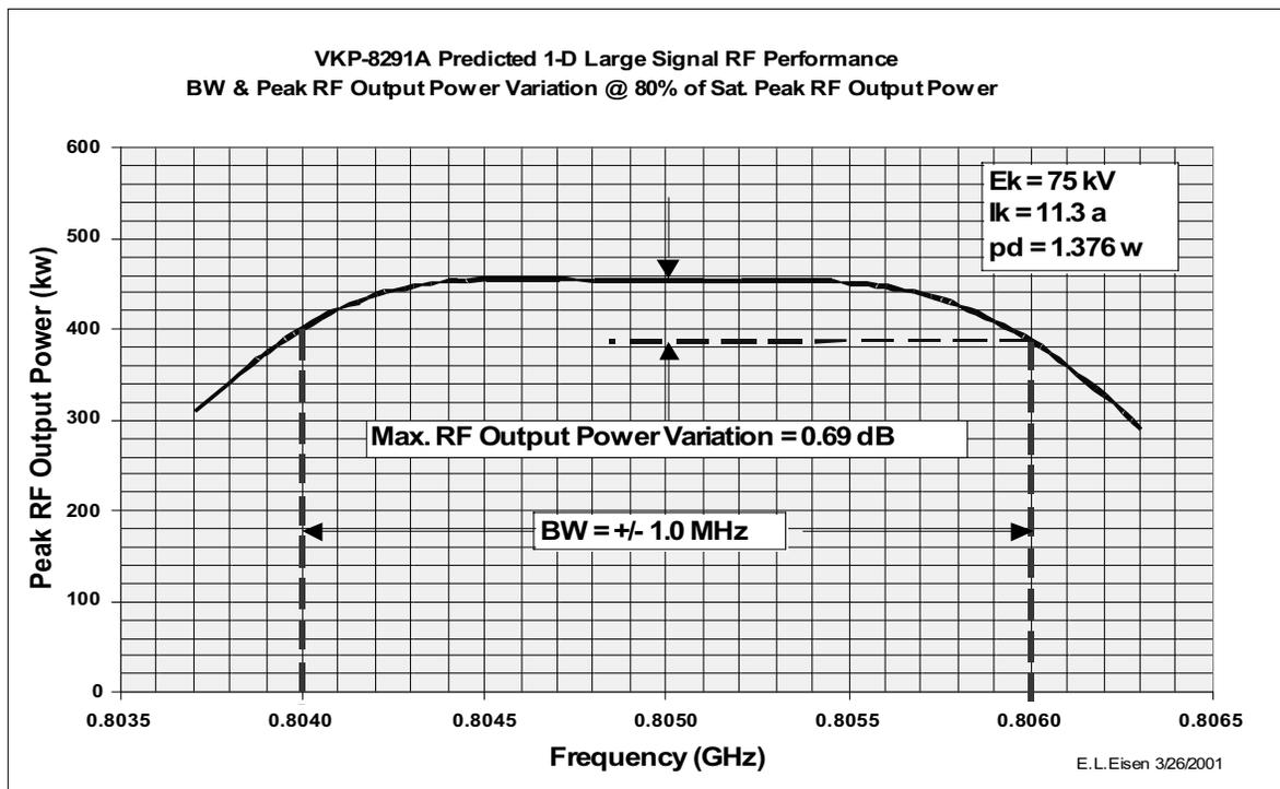
**Figure 18** – VKP-8291A Peak RF Output Power versus Frequency — Reduced Output Power Bandwidth Simulation
