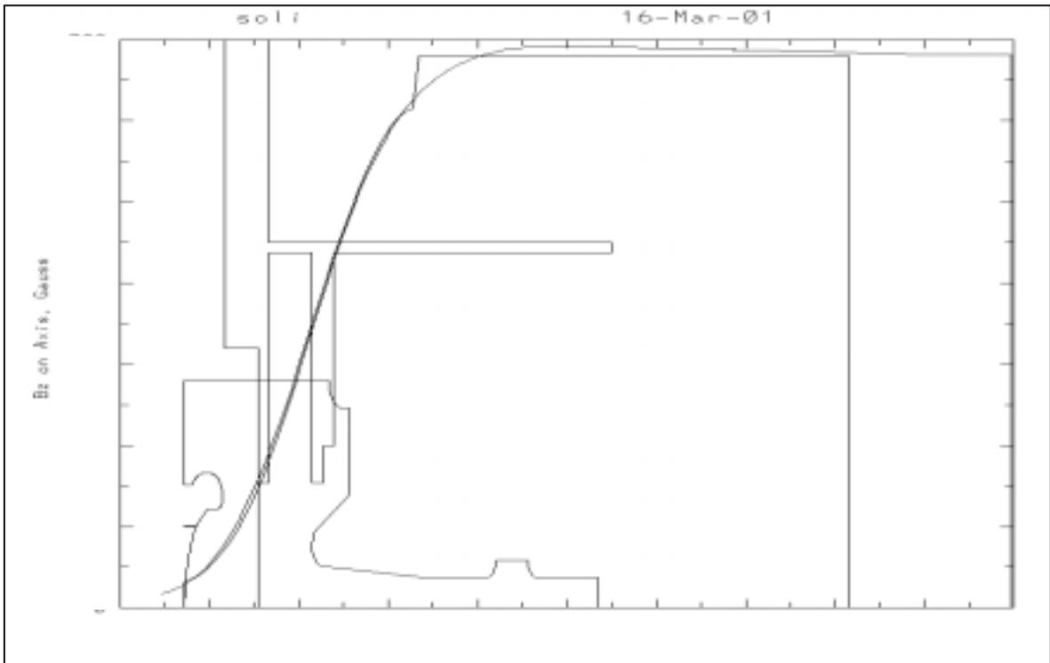
**Figure 12** – VKP-8291A Klystron – Solenoid Magnetic Field Profile in Cathode Region
