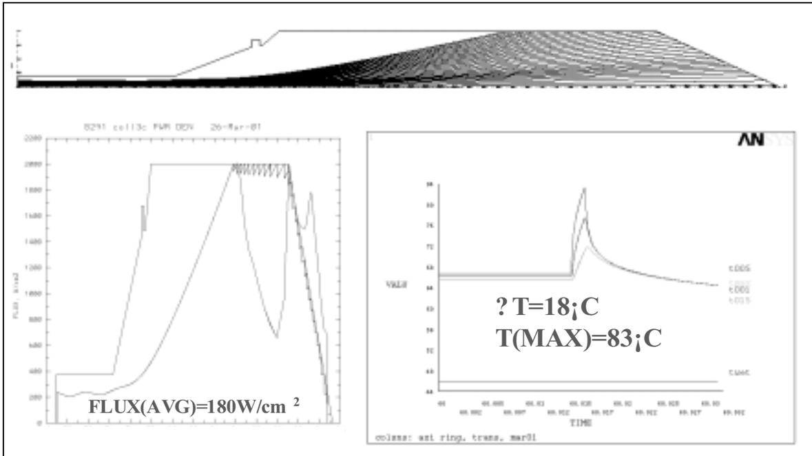
Figure 15 – VKP-8291A Klystron – Beam Simulation in Collector Region – Pulse Heating Simulation
