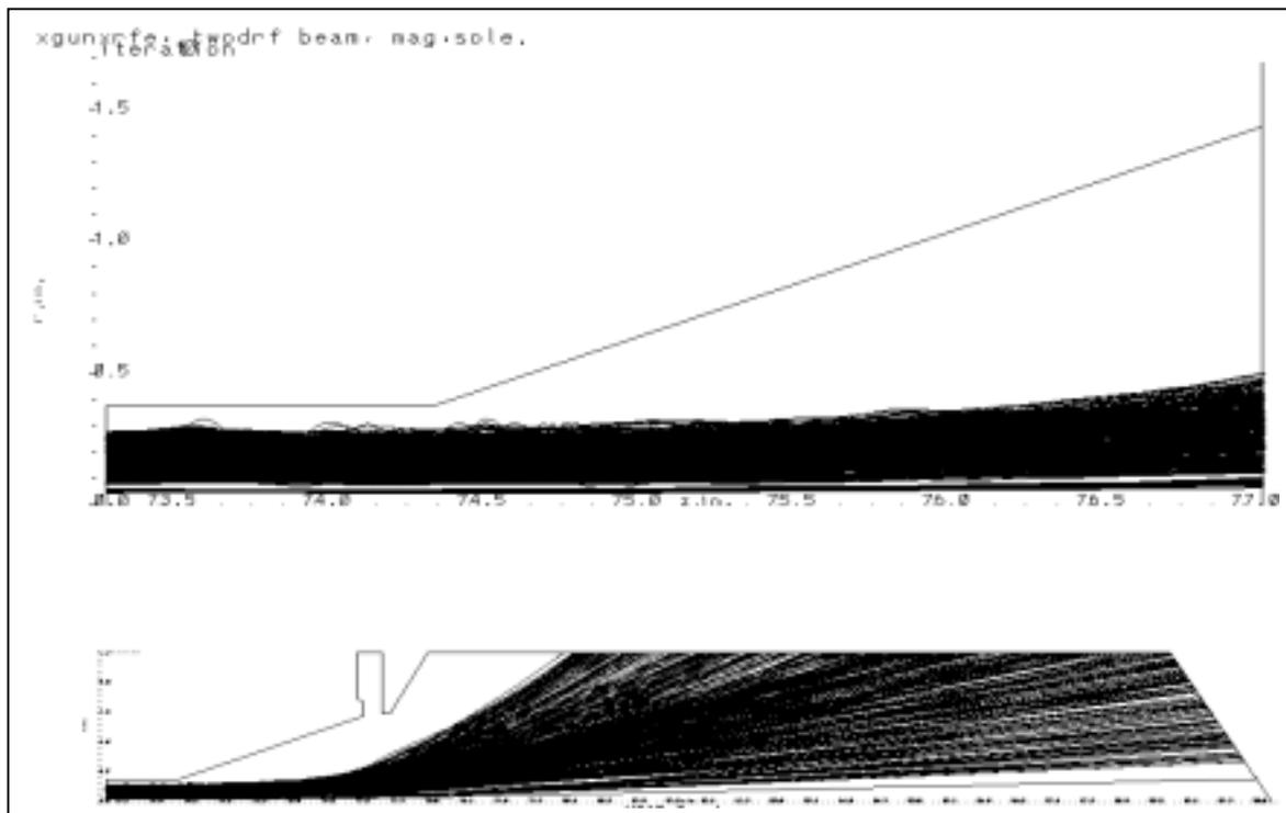
**Figure 14** – VKP-8291A Klystron – 2-D RF Beam Simulation in Collector Region
