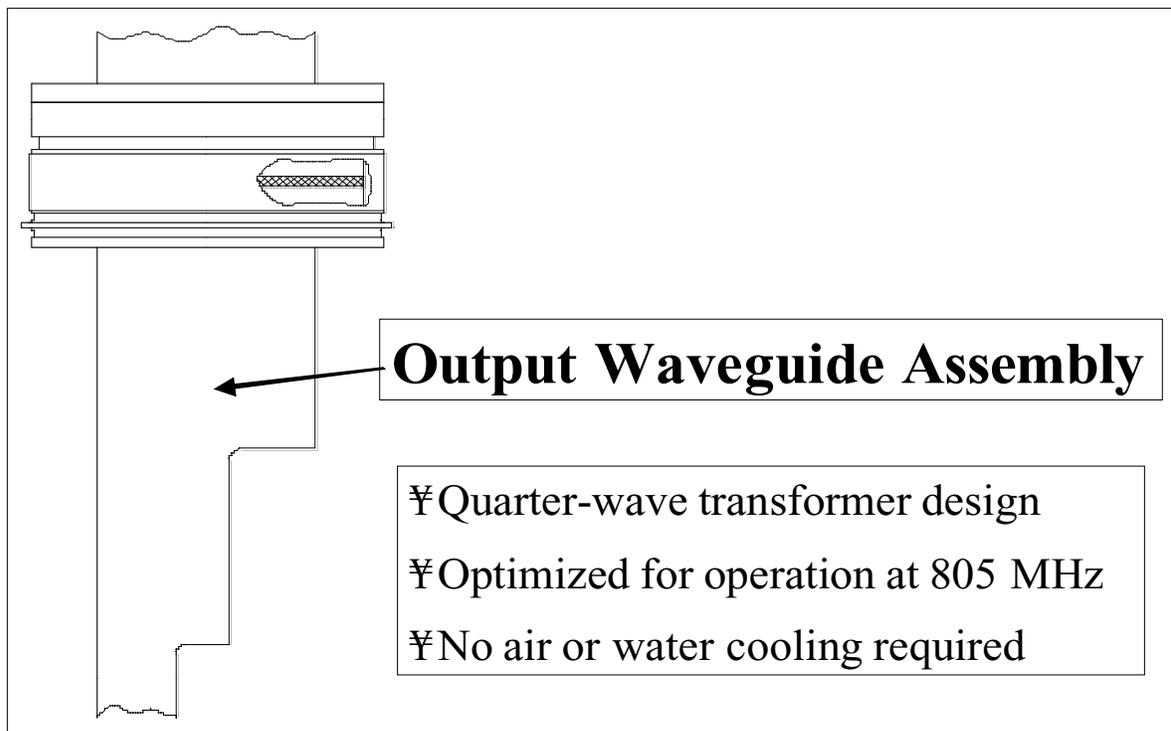
**Figure 8** – VKP-8291A Klystron – RF Waveguide Design
