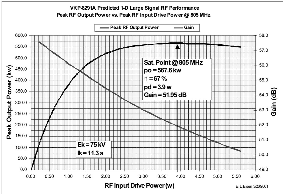
Figure 16 – VKP-8291A Peak RF Output Power versus Peak RF Input Drive Power Simulation
