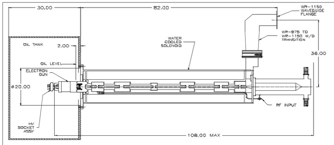
Figure 5 – VKP-8291A Klystron Layout Drawing
