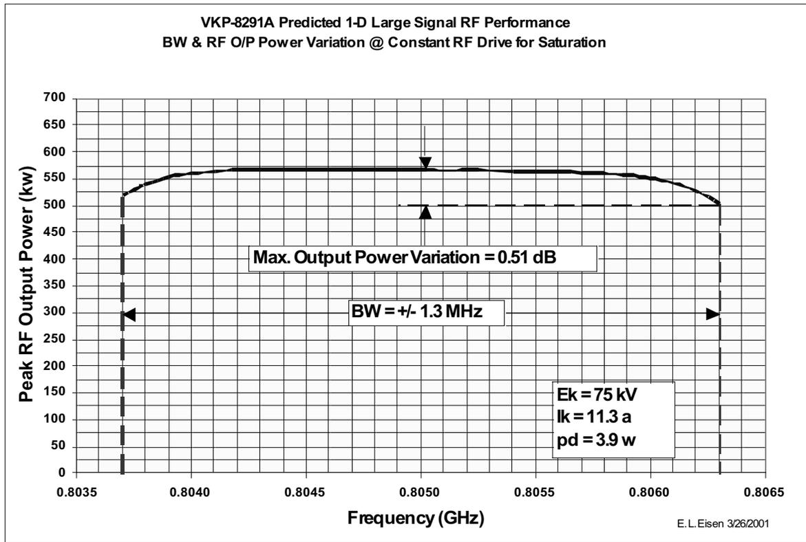
**Figure 17** – VKP-8291A Peak RF Output Power versus Frequency — Saturated Output Power Bandwidth Simulation
