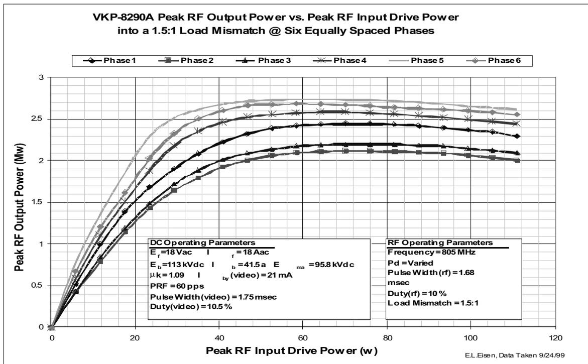
Figure 4 - VKP-8290A Peak RF Output Power versus Peak RF Input Drive Power as a Function of Load Mismatch Phase
