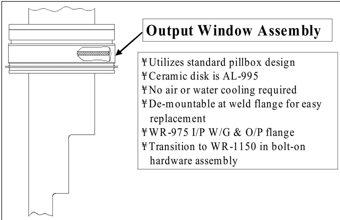
**Figure 7** – VKP-8291A Klystron – RF Vacuum Window Design
