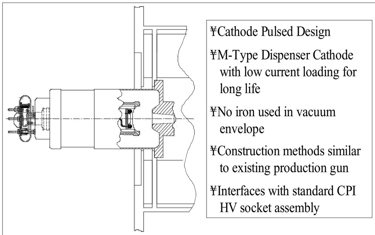
**Figure 6** – VKP-8291A Klystron - Electron Gun Design
