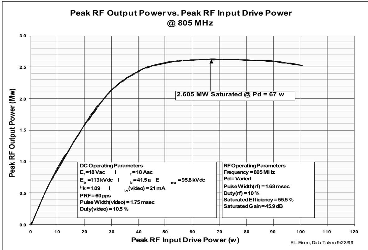
**Figure 2** — VKP-8290A Peak RF Output Power versus Peak RF Input Drive Power
