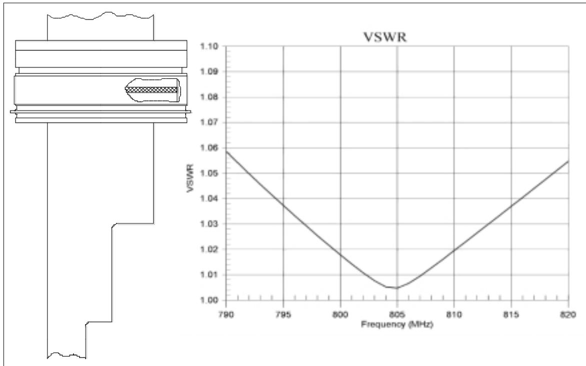
**Figure 19** – VKP-8291A RF Vacuum Window and Waveguide Assembly — VSWR versus Frequency Simulation
