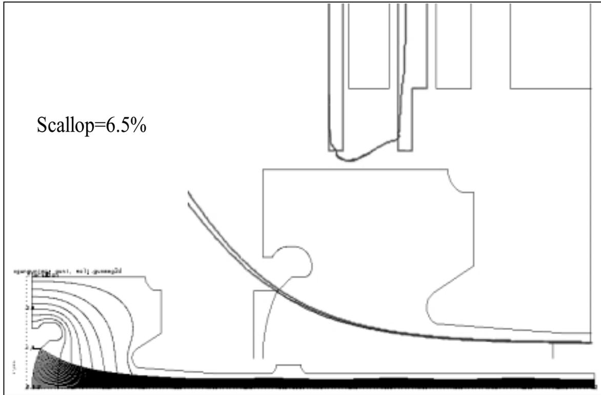
**Figure 13** – VKP-8291A Klystron – 2-D Magnetic Field Beam Simulation
