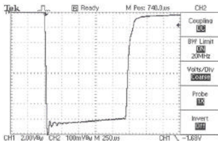
Figure 2 140 kV Output Pulse, 20 kV/Division
