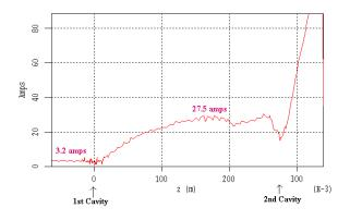
Fig. 7. RF current vs. Z.
