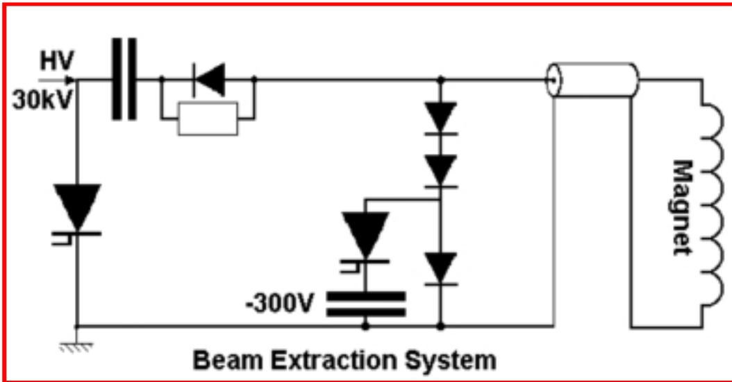
Fig. 5: Basic circuit diagram of MKD generator
