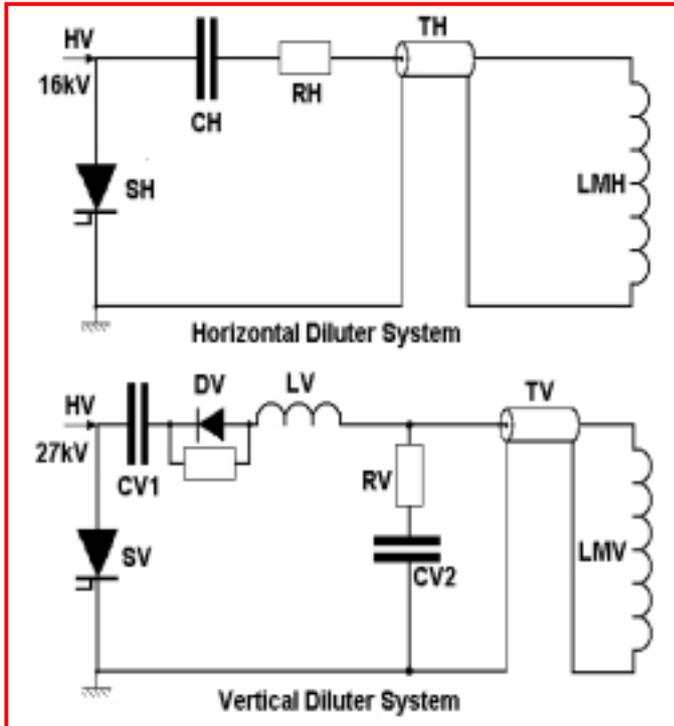
Fig. 8: Basic circuit diagram of MKB generators
