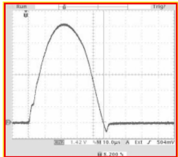
Fig. 4: MKDH switch current at 12 kV (Hor. scale 10  $\mu$ s/div., Vert. scale 4 kA/div.)
