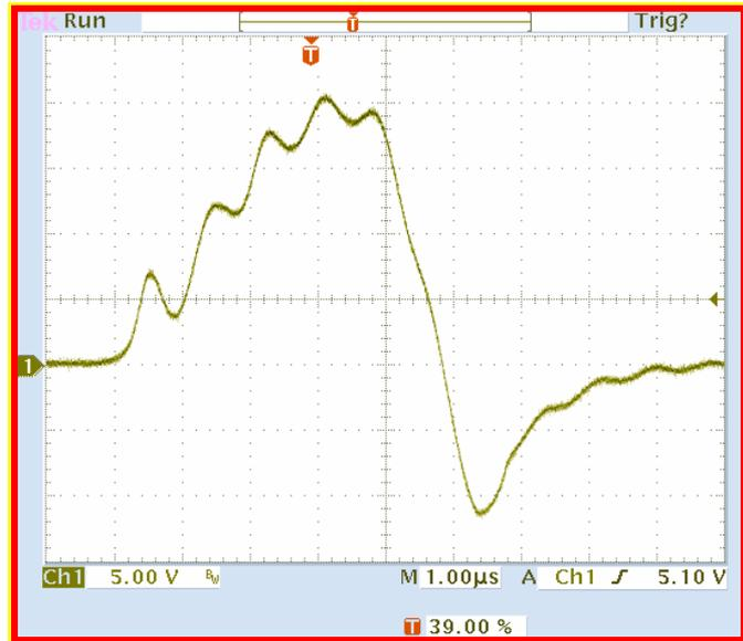
Fig. 7: MKD switch current at 30 kV
