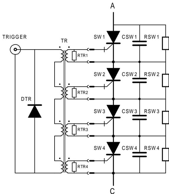
Fig. 2: Circuit diagram of MKDH switch
