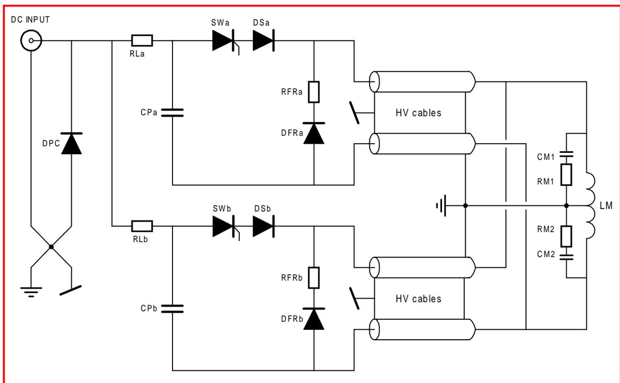
Fig. 1: Basic circuit diagram of MKDH generator
