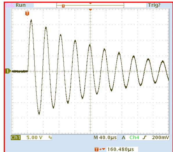
Fig. 9: MKBH test switch current (32 kA)
