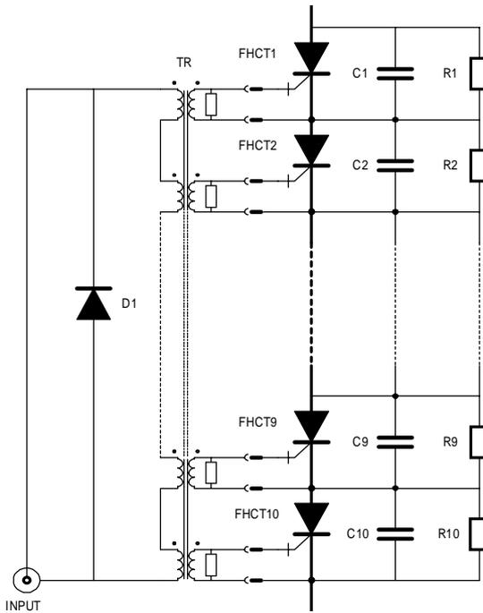
Fig. 6: Circuit diagram of MKD switch
