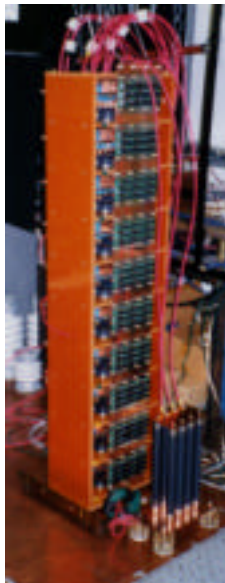
Fig. 10 10-Stage Test Modulator.
