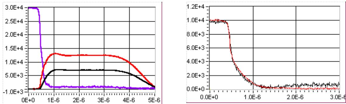
(a) Switch Voltage (V) after subtracting inductive voltage drop, load voltage(V), and load current (A).
