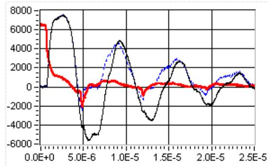
Figure 7. Load fault, 3 $\mu$ s PFN. Switch voltage, V, (bold), load current, A, and switch current, A, (dashed).
