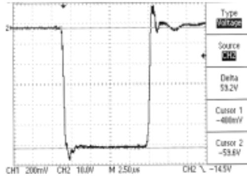
Fig. 3 60-ampere klystron current pulse from CLW modulator
