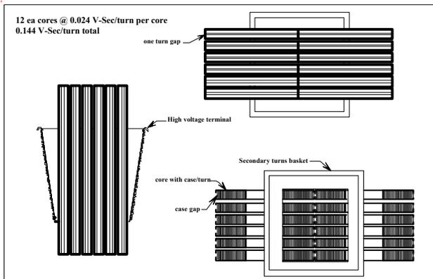
Figure 8 Pulse transformer configuration
