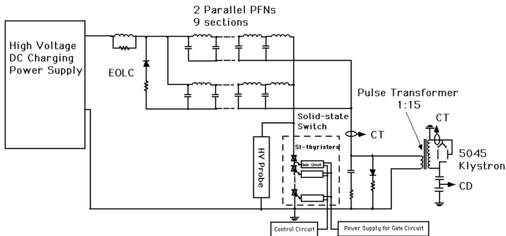
Fig. 3 Simplified circuit diagram of the klystron modulator.
