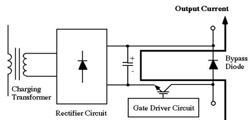
Fig. 8(b) Cell-modulator when the switch is turned on.
