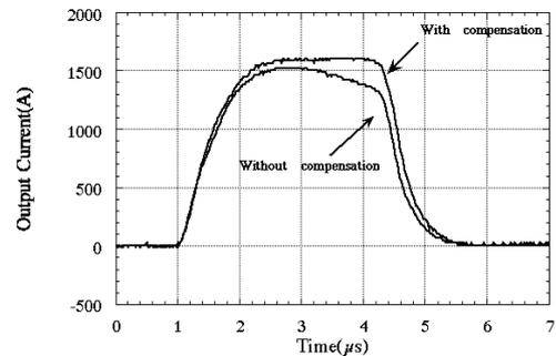
Fig. 14 Output current waveforms with and without compensation.
