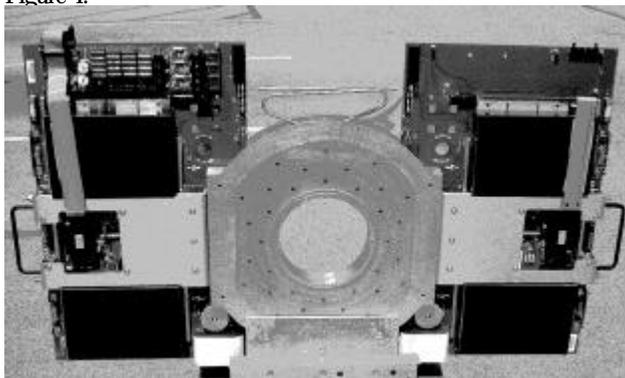
Figure 4. PC Board Core Driver circuit
