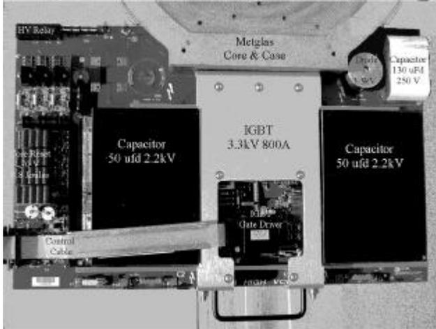
Figure 3. IGBT Drives boards
