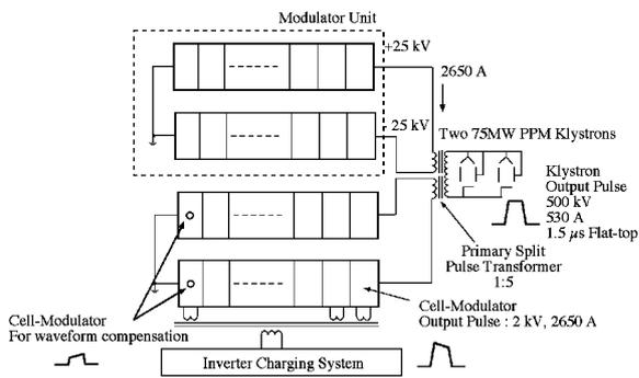
Fig. 7 Basic circuit diagram of JLC Klystron Modulator.
