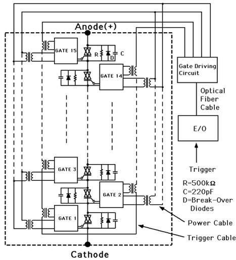
Fig. 1 Simplified circuit diagram of 45kV Solid-State Switch.
