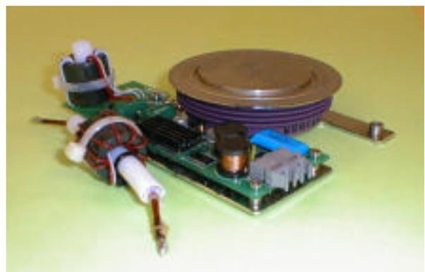
Fig. 2(b) Gate driving circuit and SI-thyristor.
