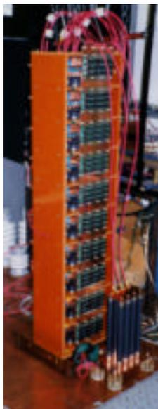
Fig. 10 10-Stage Test Modulator.
