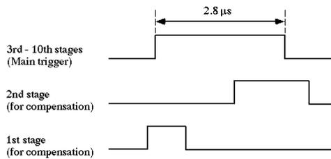
Fig. 13 Trigger timing chart.
