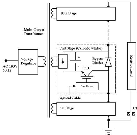
Fig. 9 Simplified Schematic of 10-stage Test Modulator Circuit.
