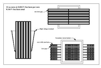
Figure 8 Pulse transformer configuration
