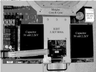
Figure 3. IGBT Drives boards
