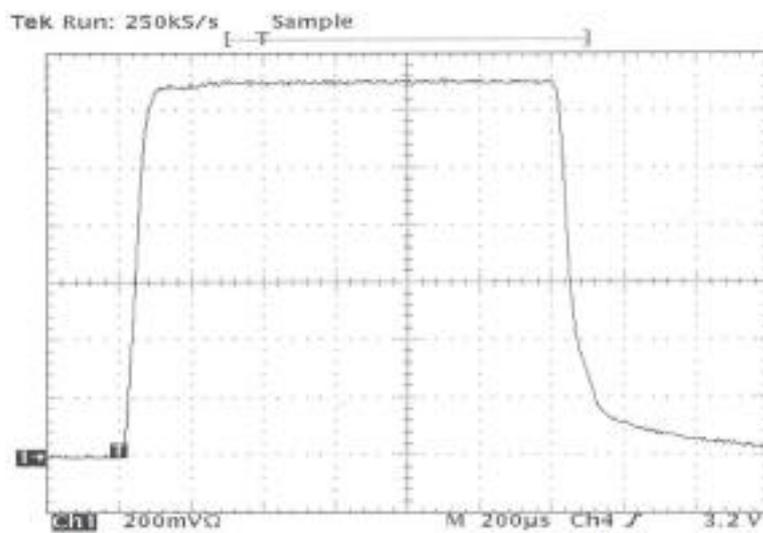
Figure 4 80 kV Output with Adaptive Feedback/Feedforward
