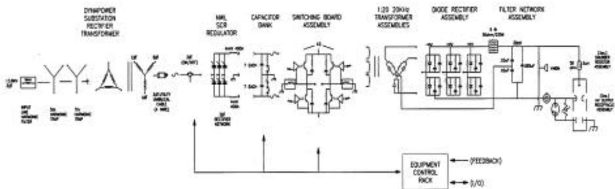
Figure 1 Simplified Block Diagram
