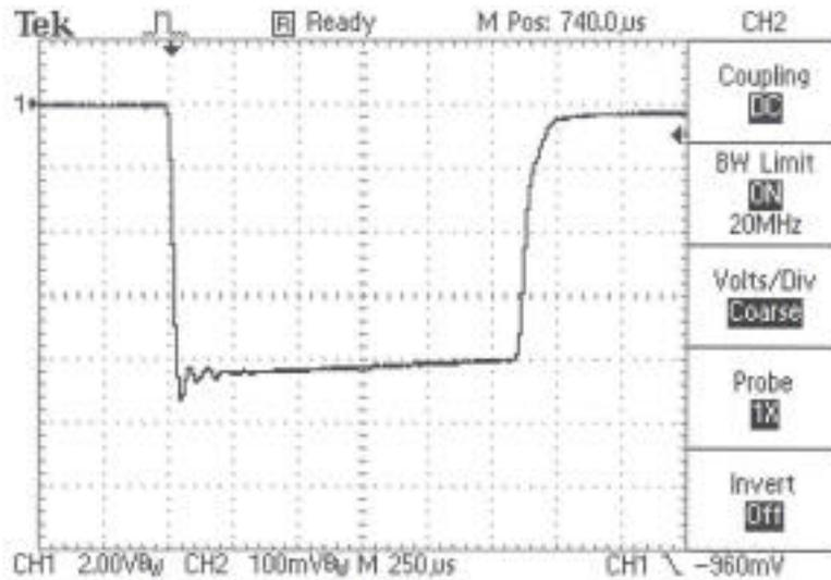
Figure 3 80 kV Output Pulse, 20 kV/Division
