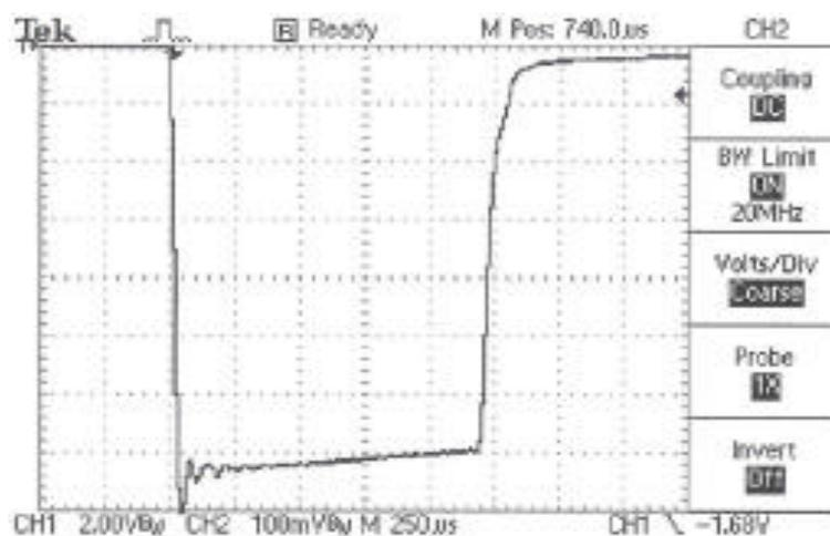
Figure 2 140 kV Output Pulse, 20 kV/Division
